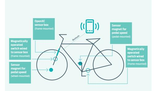
First, the electronic sensor box gathers sensor data, then the accompanying software libraries and application programming interface provide a way for developers to create custom applications and sensors.
