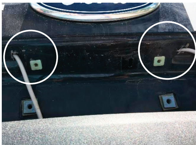
Factory-installed lights removed, with holes left uncapped. New holes added to accommodate after-market wiring.
