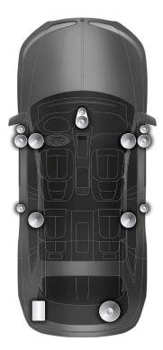
The Revel audio system for the 2016 Lincoln MKX includes QuantumLogic Surround<sup>®</sup> and 13 speakers positioned to deliver a high-quality listening experience.
