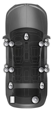
The Revel Ultima audio system for the 2016 Lincoln MKX includes QuantumLogic Surround,<sup>®</sup> Clari-Fi<sup>™</sup> technology and 19 speakers positioned to deliver an unparalleled listening experience.
